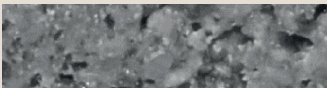
Korn an Korn Porung
